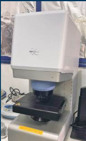
Caption: FTIR-microscope at the Hummingbird Analytical Laboratory at the University of Belize.
